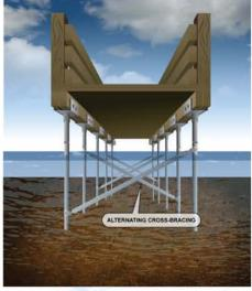
RCS (Round Corner Square) or pipe pile shafts are used depending on best fit for site conditions and for a cost effective solution. Cross bracing can be added for increase stability.
